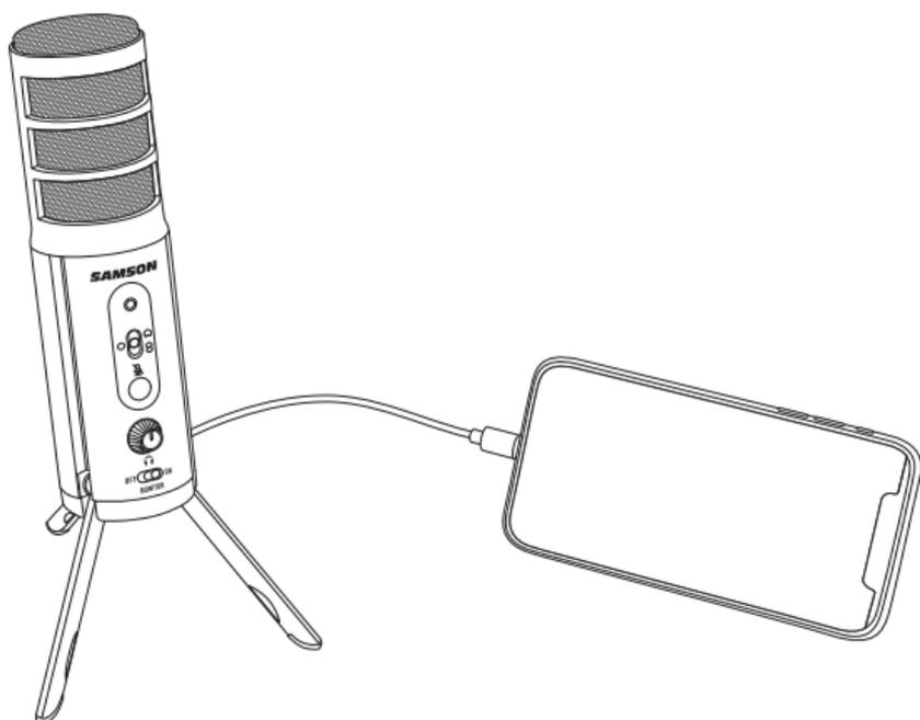
1. Connect the Satellite to an iPhone or iPad using the included USB to Lightning cable.
